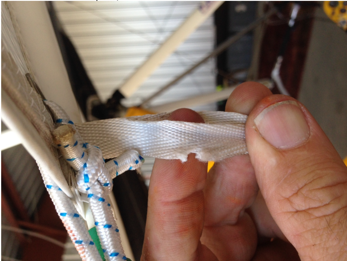
Fig 1 example of damaged webbing when removed from the eyelet.
