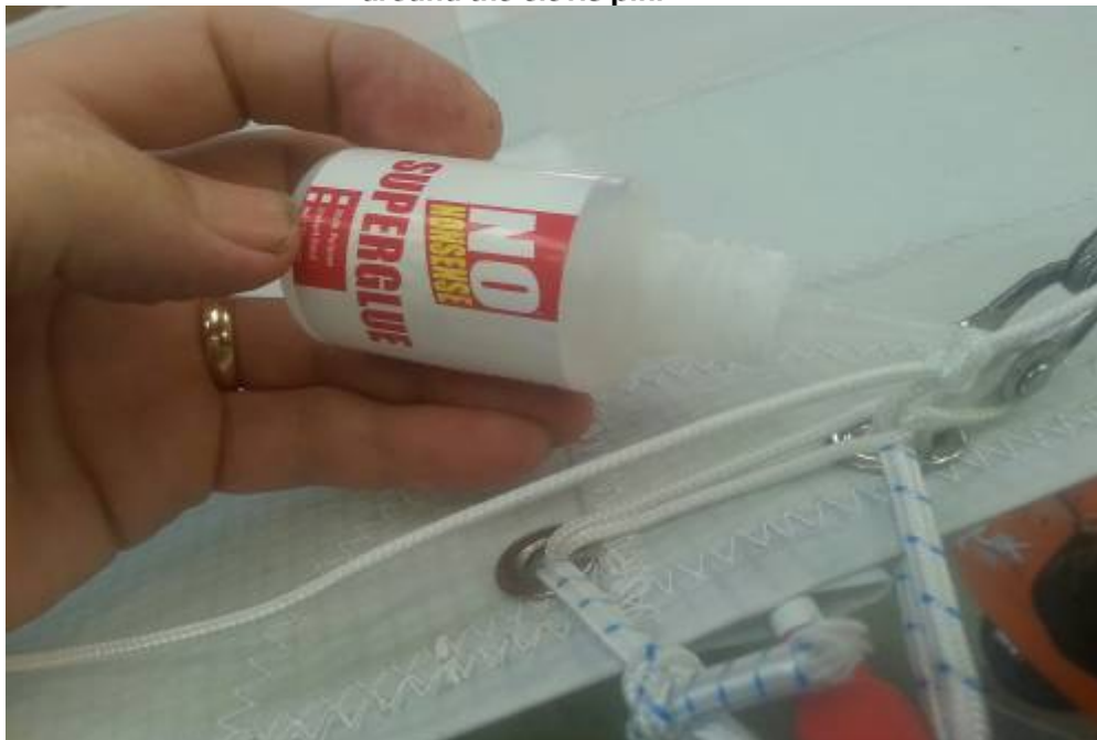
Fig 5 loop the cord through both eyelets, tie the ends off around the clevis pin with a reef knot. Use pliers to get it really tight. Apply cyanoacrylate to the knot ( superglue). . Note there should be no slack in the cord.
