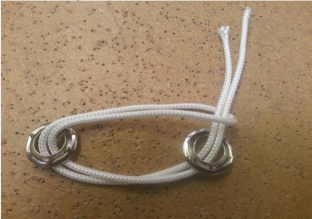
Fig 4 showing the cord loop and the routing through the eyelets. The free ends are tied around the clevis pin.
