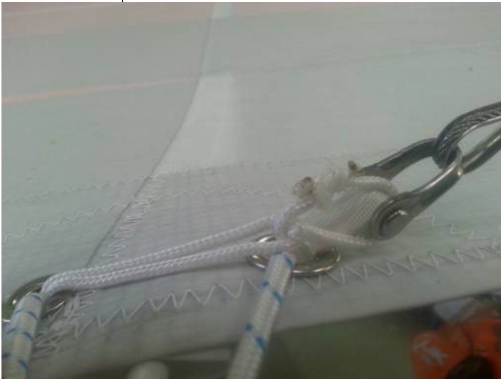
Fig 6 cut and seal the ends of the cord using a hot knife or soldering iron.
